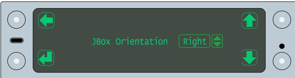
4. Tap the scroll up or scroll down button until the correct orientation option is displayed
