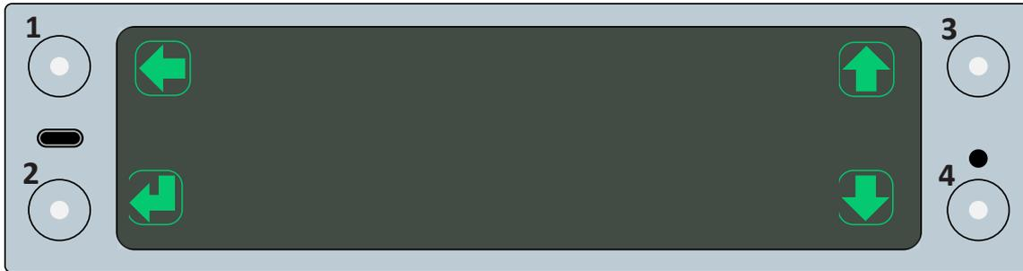
Each touch pad is illuminated by LED. It can be tapped to activate the corresponding action on the screen next to it.
