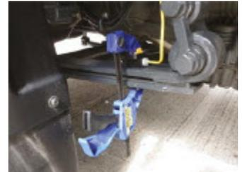
Use cable protector to protect the cable at positions where it may be exposed to damage
