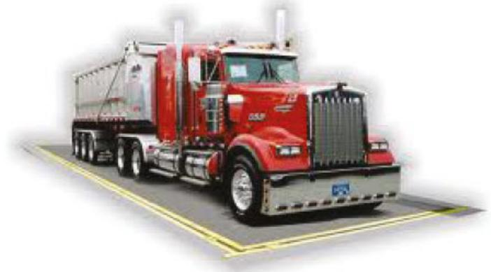
5. Drive the vehicle off the weighbridge, one axle at a time. Take the weight measurements until you have a value for each time an axle is removed from the weigh bridge
