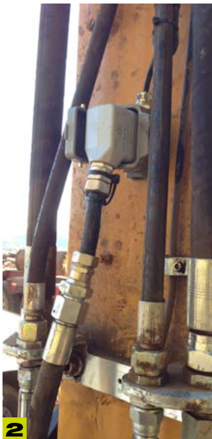
Heavy duty quick disconnect plug installed on the stick
