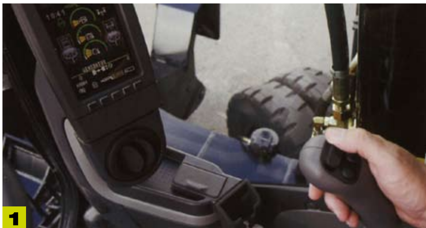
Totalizing option with push button using the machine lever free one
