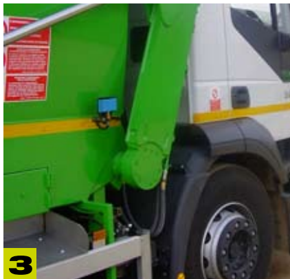
Contactless weighing zone sensor for weight reading
