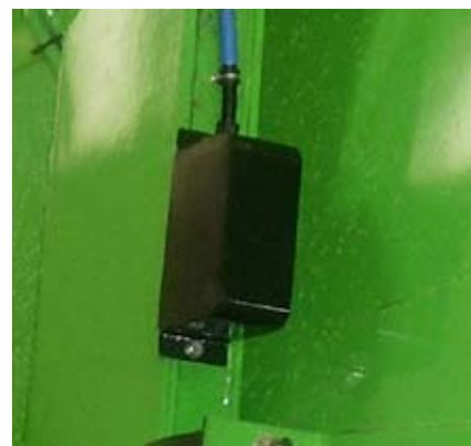
Contactless weighing zone sensor for weight reading
