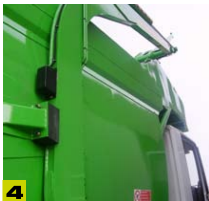
Load sensors, one each arm
