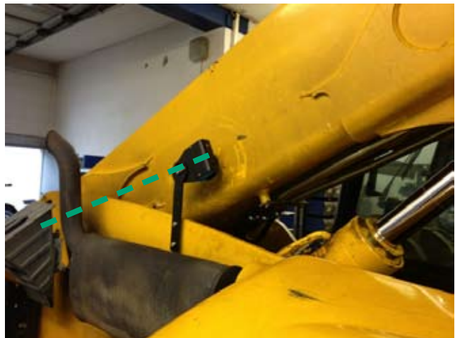
Fig. 2 Weighing Zone sensor position in line with boom's pin
