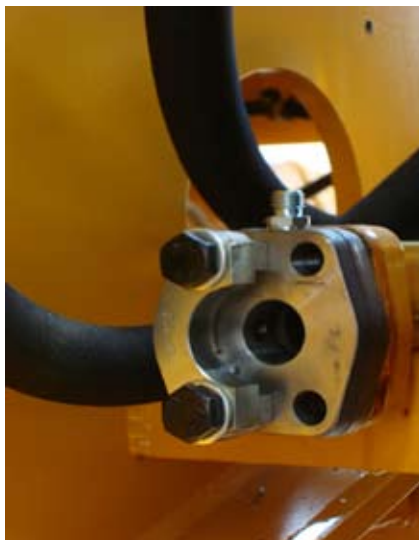
Fig.3 Vei flange fitting install
