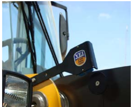
Fig.2 Weighing Zone bracket position
