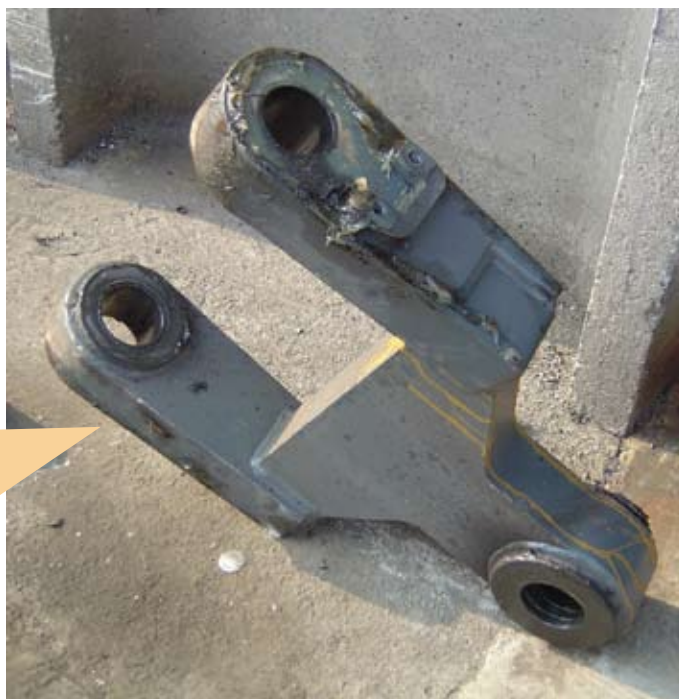
Fig.2 Original Yoke uninstalled
