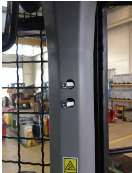
Fig.13 Cat 924K pilar with plastic cover
