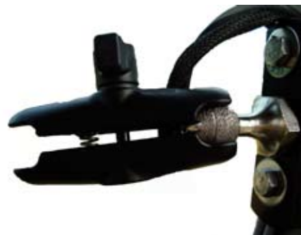
Fig.1 Device Bracket fixed onto the cabin pillar
