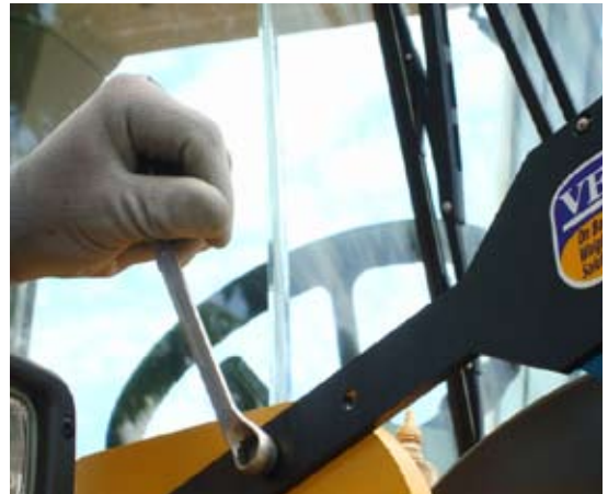
Fig.5 Tapping Weighing Zone bracket fixing points
