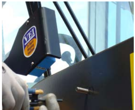
Fig.11 Installing Weighing Zone reference headless screw
