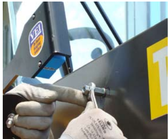
Fig.12 Installing Weighing Zone reference hexagon
