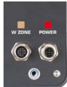
Fig.2 Device with M12 connectors. Weighing button is connected to W.zone
