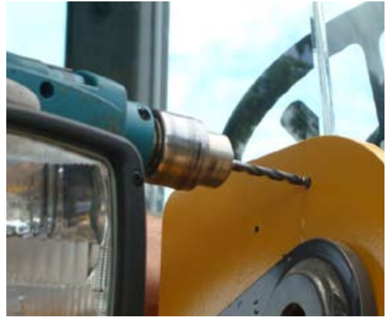
Fig.3 Drilling Weighing Zone bracket fixing points
