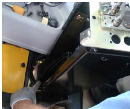
Fig.3 Harness entering the cabin from top
