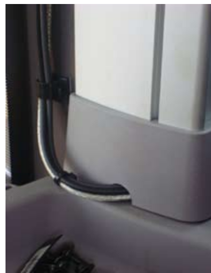
Fig.4 Harness fixed onto the pillar
