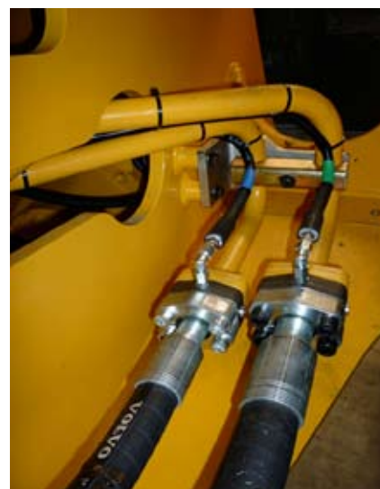
Fig.6 Sensors fitted into Vei fitting
