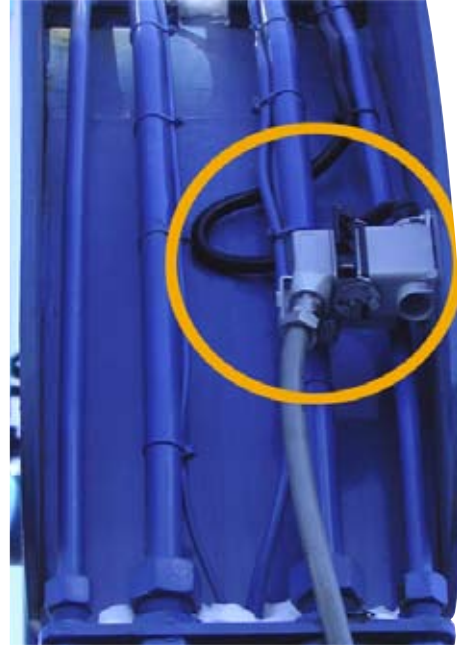
Fig.5 Quick disconnect plug onto the stick boom
