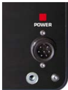
Fig.1 Device with AMPHENOL connectors. Weighing button is connected to Power
