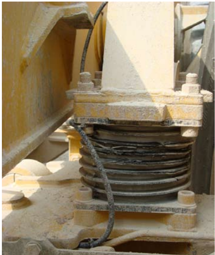
Fig.1 Load Link wiring towards the cabin
