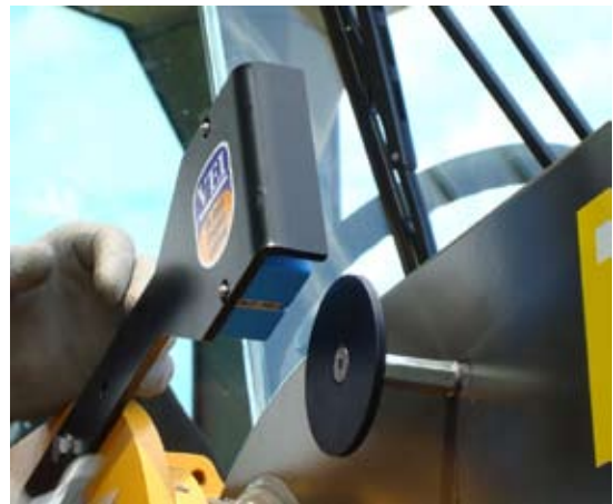
Fig.13 Weighing Zone reference disk
