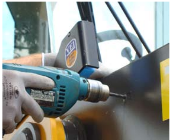
Fig.9 Drilling Weighing Zone reference fixing point
