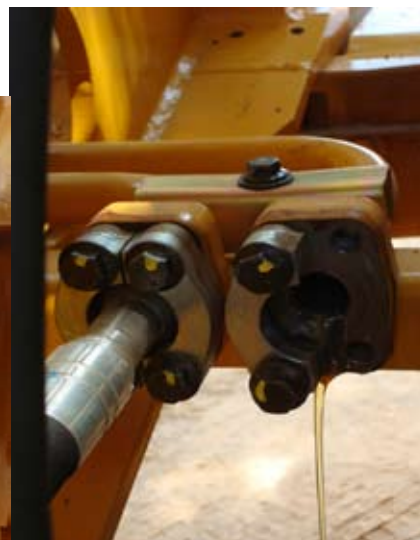
Fig.1 Original fitting removal
